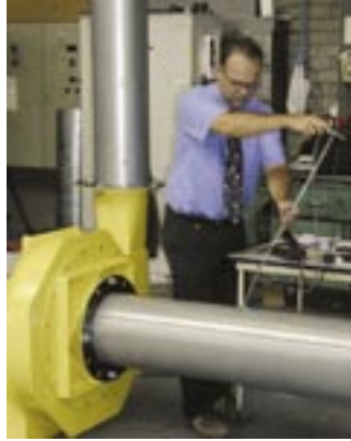
Capacity measuring fan in the R & D department.
