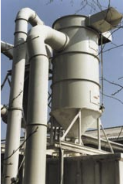
Compressed air-cleaned bagfilter type Cobra-Jet with the production of wood-wool cement plates.
