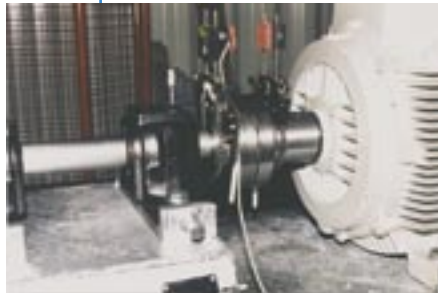
Alignment-adjusting of a coupling with laser equipment.
