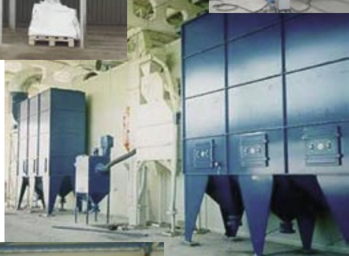
Bag filter type SMKT-225 for the exhaust of a blasting hall for railwaycoaches. Total exhaust-capacity: 81,000 m 3 /h.
